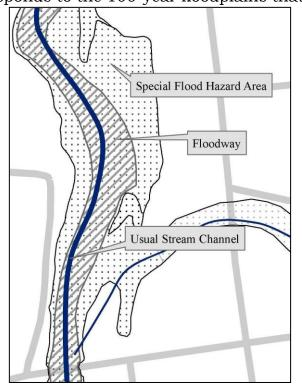
surface elevation (usually areas of ponding) where average depths are between 1 and 3 feet. The BFEs derived from the detailed hydraulic analyses are shown at selected intervals within this zone. The extent of floodways may be shown on separate map panels in communities that have established BFEs.
